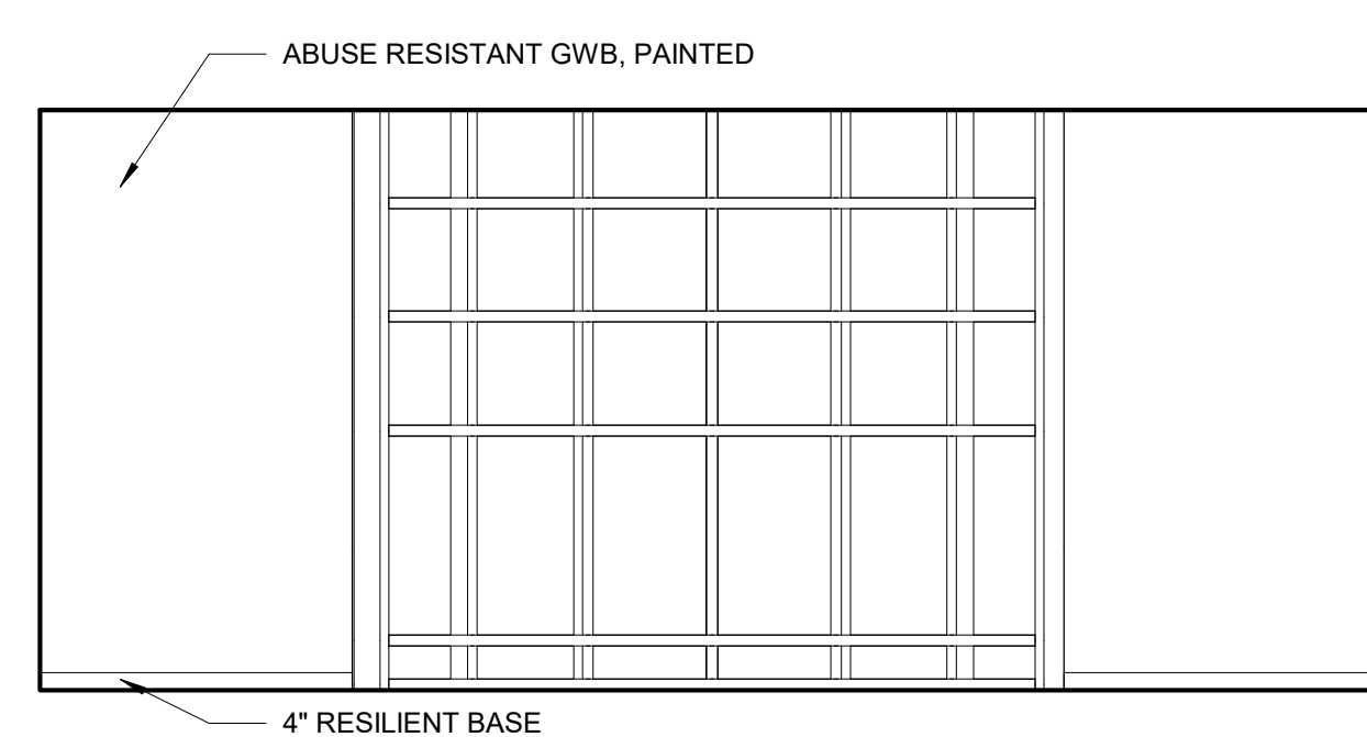
3 TYPICAL CLASSROOM ELEVATION 1/4" = 1'-0"
