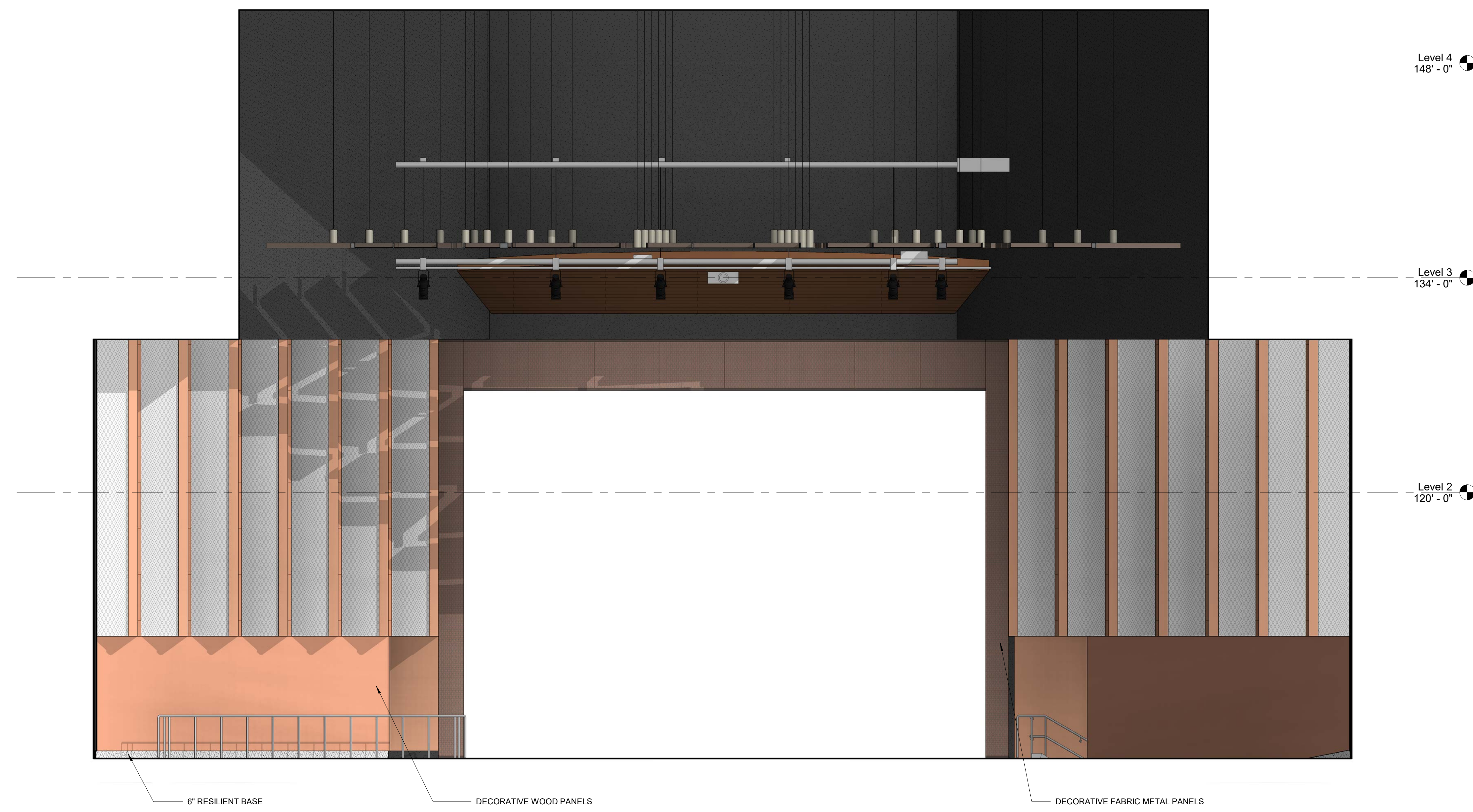
2 AUDITORIUM INTERIOR ELEVATION 1/4" = 1'-0"
