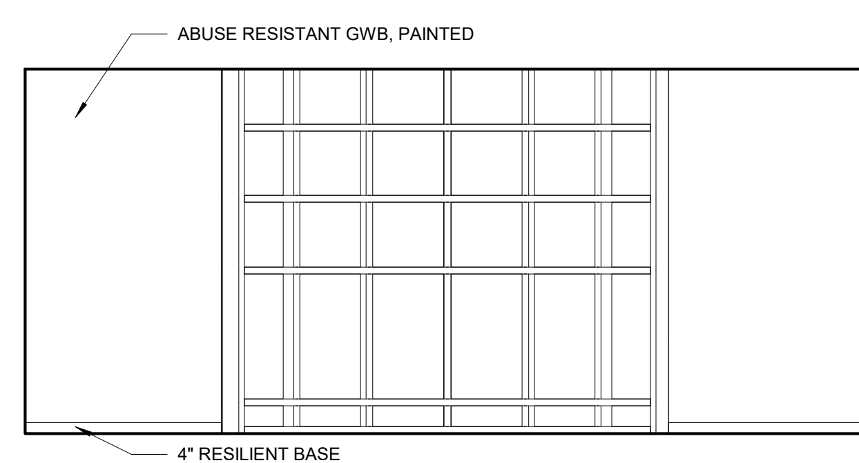
3 TYPICAL CLASSROOM ELEVATION 1/4" = 1'-0"
